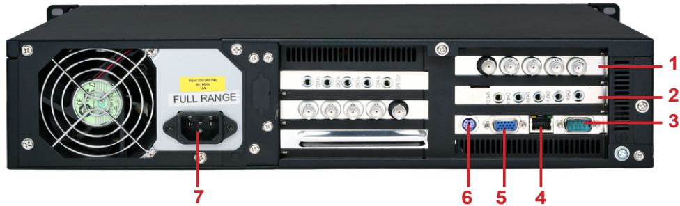
1. Video-In×4 (optinal) 2. Line In × 4 (optional) 3. COM 4. Ethernet 5. VGA 6. PS/2 7. Power Connector
