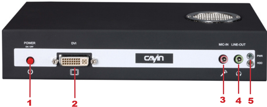
1. Power Button 2. DVI Connector 3. MIC-IN (Reserved) 4. Audio-out 5. PWR/HDD Indicator
