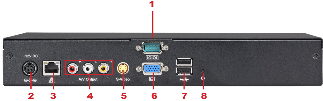
1. RS-232 2. Power Connector 3. Ethernet 4. AV-out 5. S-Video Out 6. VGA Connector (Output) 7. USB Connectors 8. Power Switch
