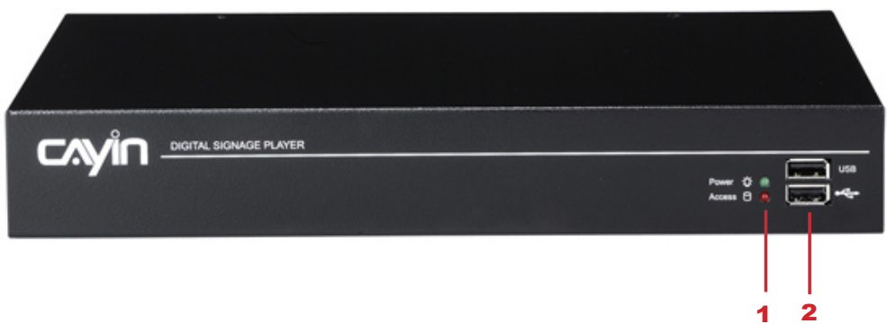
1. Power & HDD Indicators 2. Front USB Connectors
