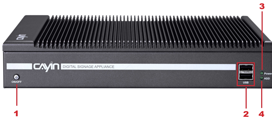
1. Power 2. USBx2 3. Power Indicator 4. Hard Disk Indicator
