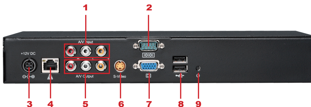
1. AV-in 2. COM Port 3. Power Connector 4. Ethernet 5. AV-Out 6. S-Video Out 7. VGA Connector (Output) 8. USB Connectors 9. Power Switch
