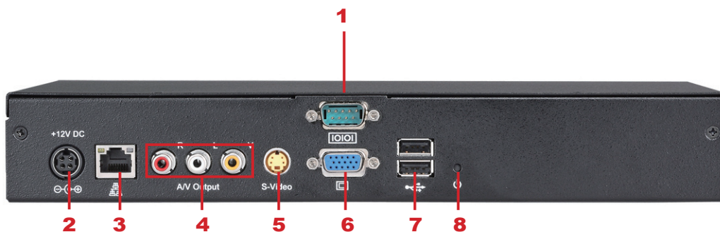
1. COM Port 2. Power Connector 3. Ethernet 4. AV-Out 5. S-Video Out 6. VGA Connector (Output) 7. USB Connectors 8. Power Switch
