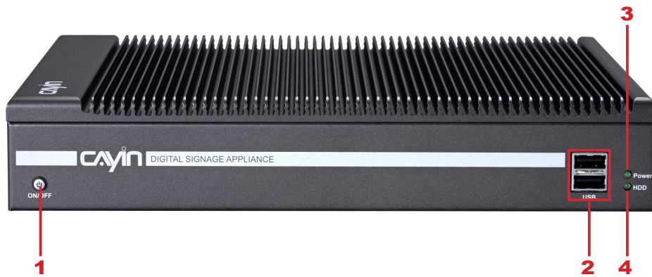
1. Power 2. USBx2 3. Power Indicator 4. Hard Disk Indicator
